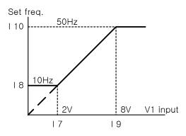
• Frequency setting via 0 ~ 10 [V] input or Terminal Potentiometer
