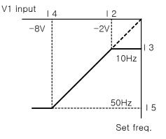
▶ I6 ~ I10: Setting input range and corresponding frequency to 0 ~ +10V V1 input voltage
