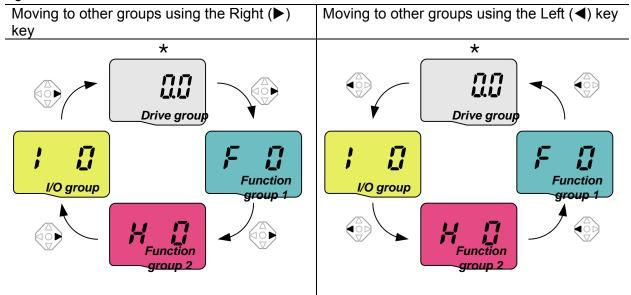
\* Target frequency can be set at **0.0** (the 1<sup>st</sup> code of drive group). Even though the preset value is 0.0, it is user-settable. The changed frequency will be displayed after it is changed.
