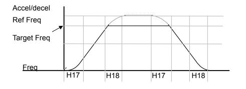
If Target Frequency is below Max Frequency, the waveform will be shown with the top portion cut out.
