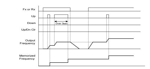
When F65 is 2: It is increased as many as step frequency set as F66 at the rising edge of multifunction input set as UP and if it is activated for 3 second, it operates like something set as "0". It is decreased as many as step frequency set as F66 at the rising edge of multi-function input set as DOWN and if it is activated for 3 second, it operates like something set as "0" and the accel/decel time is same with when stetted as "0".
