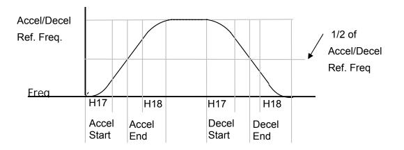
Note that setting Frequency Ref. for Accel/decel (H70) is set to Max Freq and target freq is set below Max freq. the shape of S-curve may be distorted.
