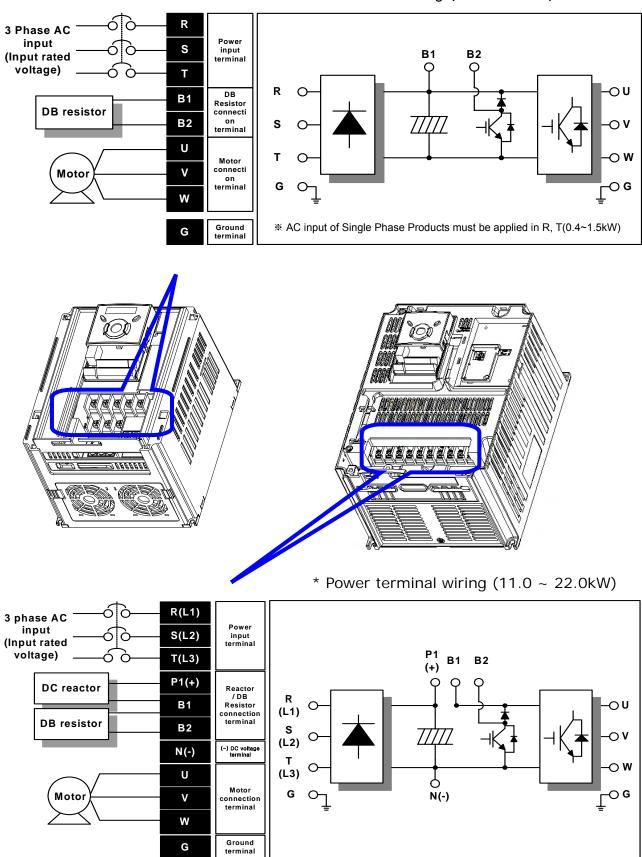
\* Power terminal wiring (0.4 ~ 7.5kW)
